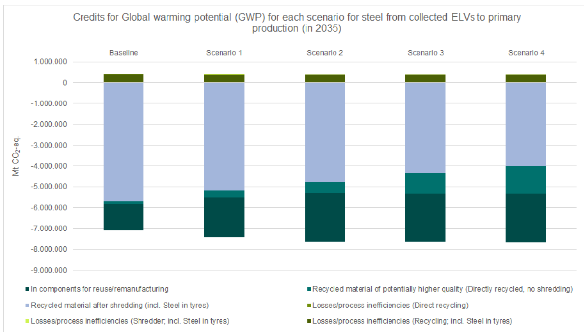
Figure 3-3 Credits for Global warming potential (GWP) for each scenario for steel in collected ELVs in 2035 to primary production (Mt CO 2 eq)
