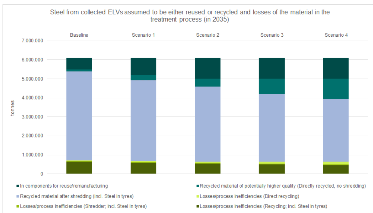
Figure 3-2 Tonnes of steel from collected ELVs assumed to be either reused or recycled and losses of the material in the treatment process (in 2035)
